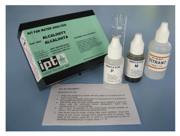
Code N° 1002 IPT ALCALINITY (phenolphthalein and methylorange alkalinity in french degrees)
